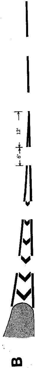
Mark No. 114 Chevron markings at approach to islands "A" Diverging traffic "B" Merging traffic.
